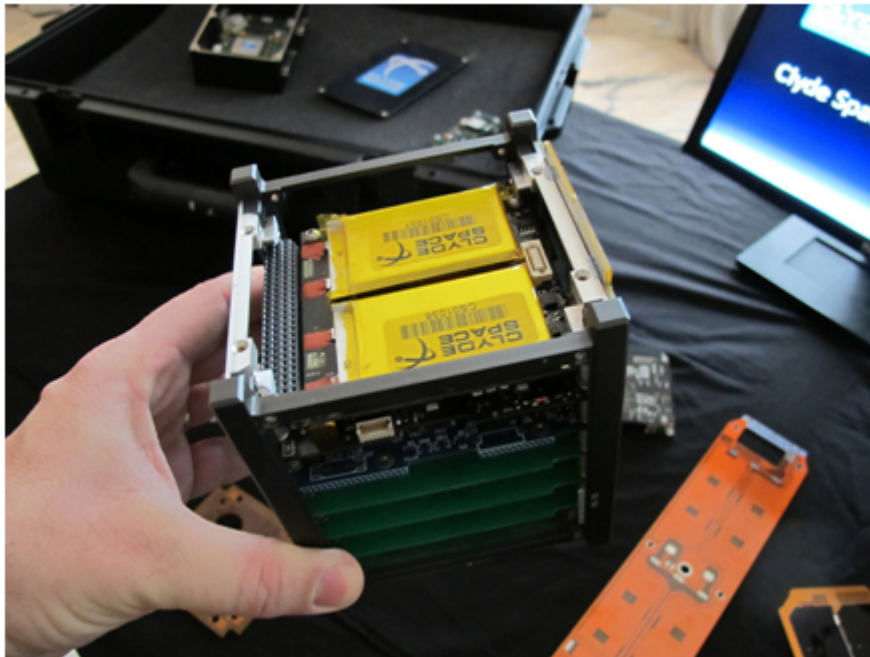
Image 1. 1U cubesat structure without outer skin (source: Wikimedia Commons user Svobodat, "1U cubesat structure without outer skin," Wikimedia Commons , 26 January 2011, https://commons.wikimedia.org/wiki/File:CubeSat_in_hand.jpg accessed 31 March 2016. Photo in public domain.)
